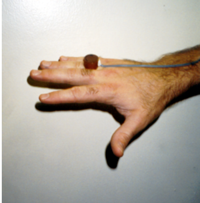
FIGURE 6: ring-mounted vibrotactile stimulator
