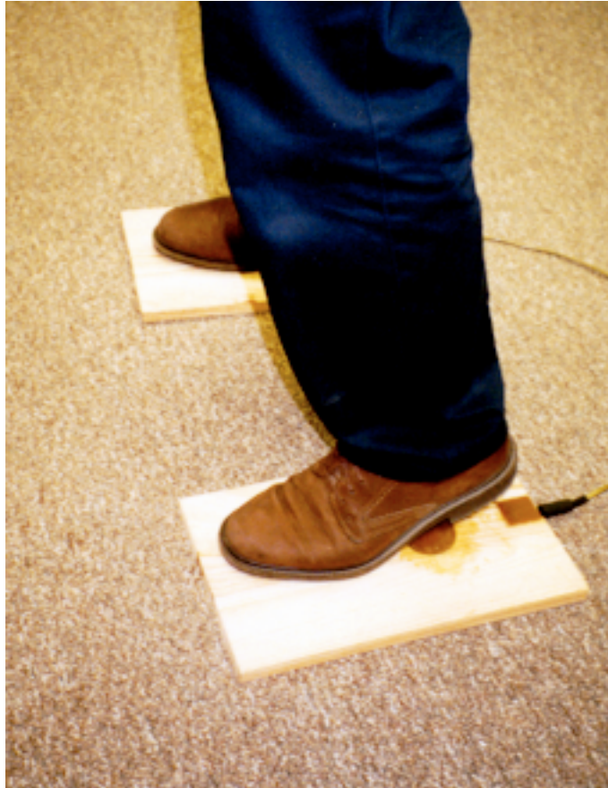
FIGURE 7: foot-sensed vibrotactile stimulator (foot raised to show stimulator)
